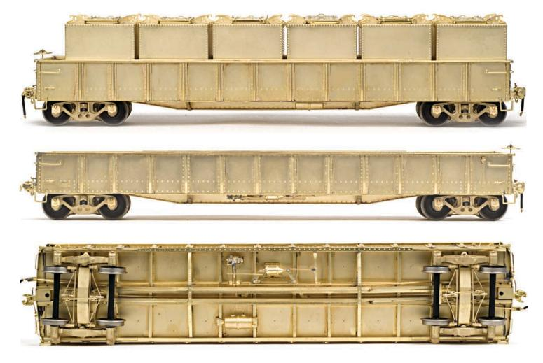
In the photos above you see elevation views of the car both with and without its container load. The containers that are shown in the photo are HB1a hopper-bottom versions. Also shown is the underside which lets you see the complete construction and running gear detail.
